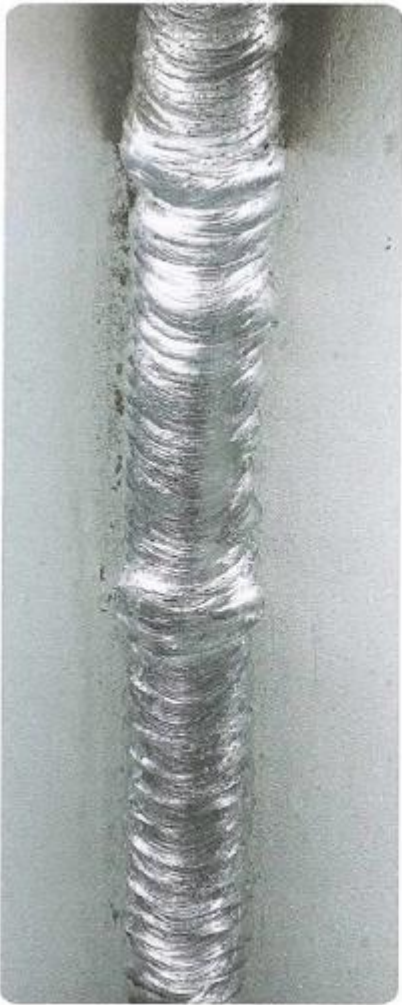
MMA: Typical good appearance of a vertical-up weld.
