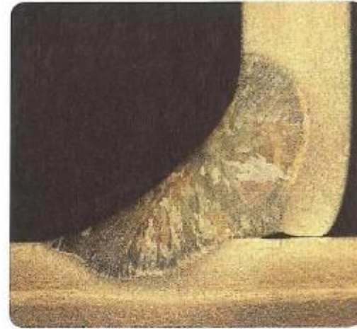
Good concave TIG fillet weld.
