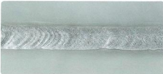
TIG: Good, clean and smooth weld.
