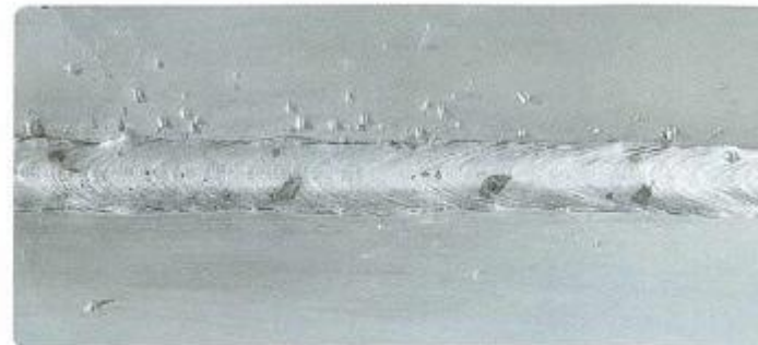
MAG short arc: Imbedded slag in the weld and spatter on the parent metal.
